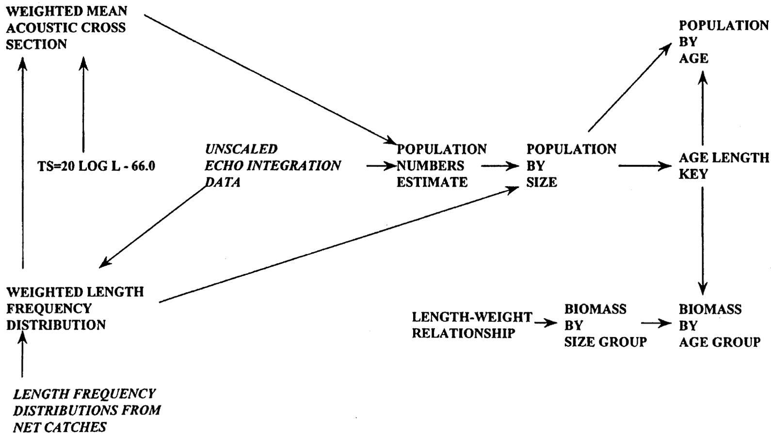
Figure 3. Schematic representation of procedure for estimating walleye pollock abundance using echo integration and net catch data. Italicized blocks are data that are measured during the survey. The remaining blocks are calculated.
