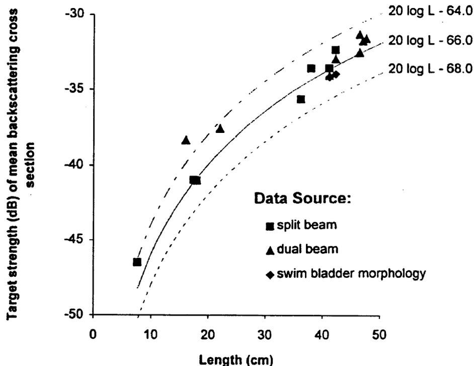
Figure 2. Target strength-to-length relationship for walleye pollock (*Theragra chalcogramma*).
