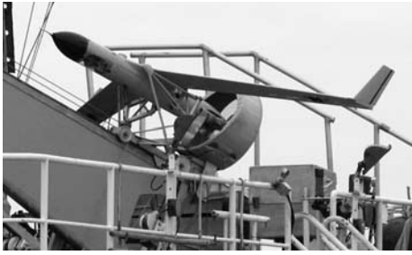
Figure 5. ScanEagle unmanned aerial aircraft system (UAS) ready for launch with propeller guard in place.
