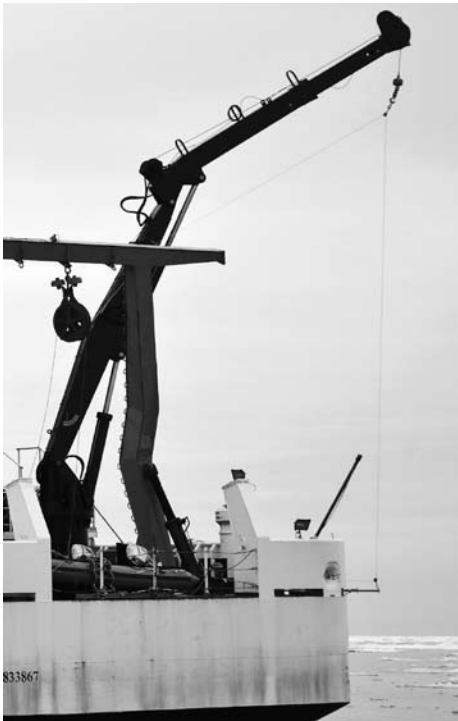
Figure 6. The SkyHook recovery system is composed of a line suspended between the ship's crane and a lower boom.
