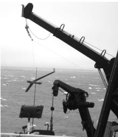
Figure 7. ScanEagle UAS about to capture the SkyHook line for recovery.
